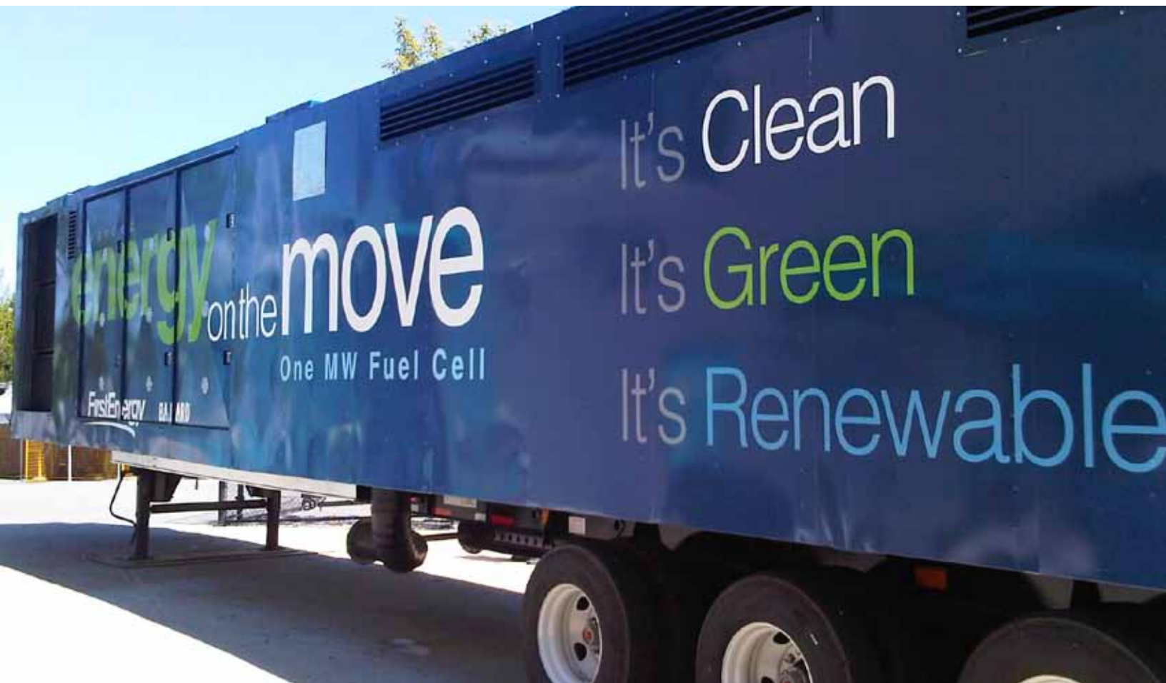
Ballard ClearGen 1 MW stationary fuel cell unit
